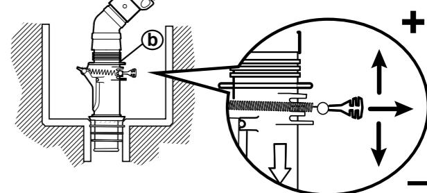
**9 Adjust flow if necessary using Flow Keeper™ Valve (b) or the valves at the equipment pad.**
